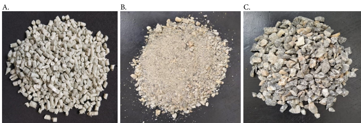
Figure 2. Waste polypropylene (A) and aggregates used: stone dust (B) and gravel (C)
