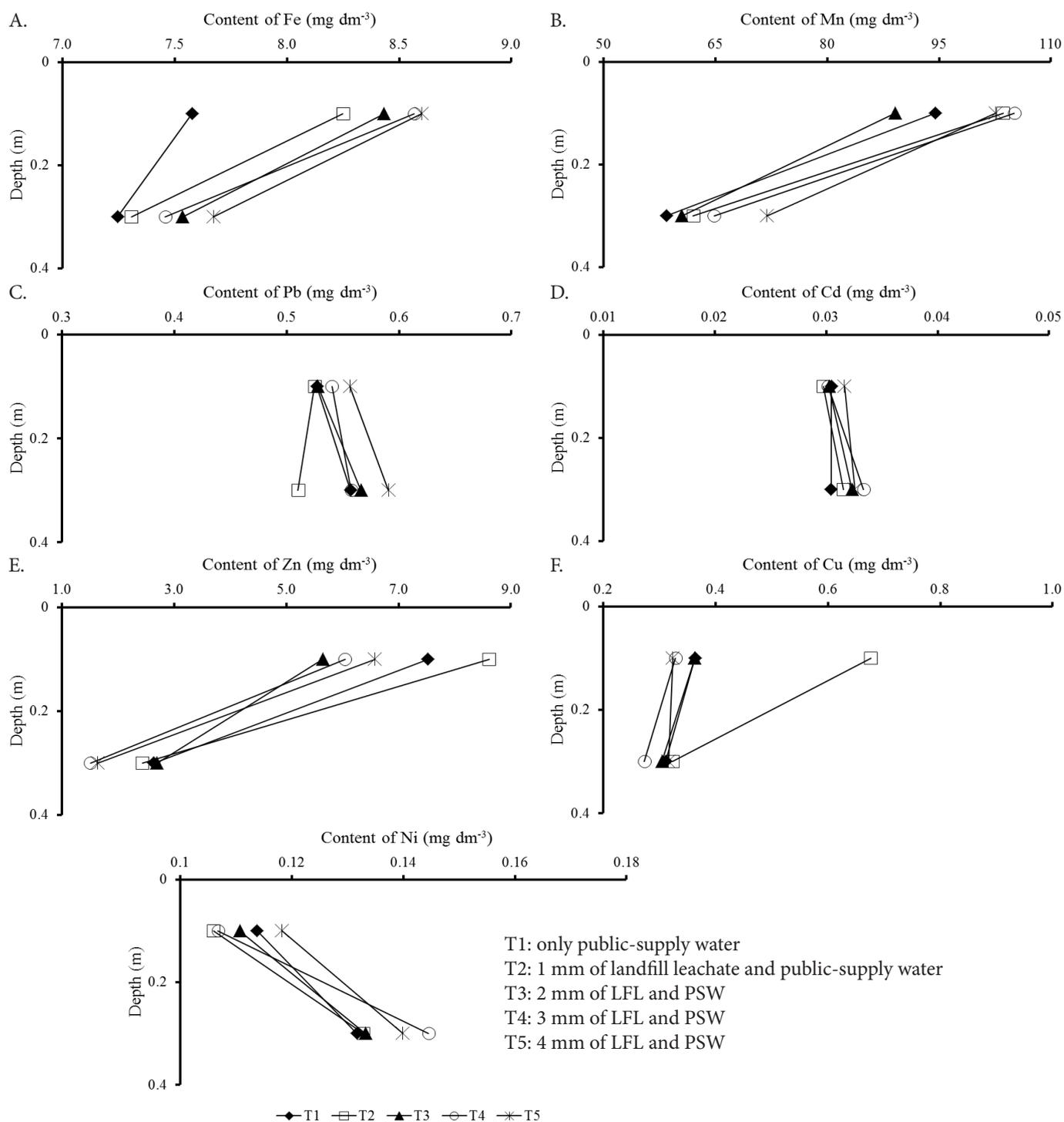
Figure 1. Behavior of Fe, Mn, Pb, Cd, Zn, Cu and Ni as a function of soil depth and treatments
