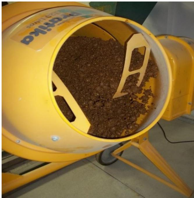
Figure 1. Mixture homogenized in concrete mixer
