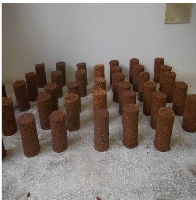
Figure 2. Specimens healing in open air
