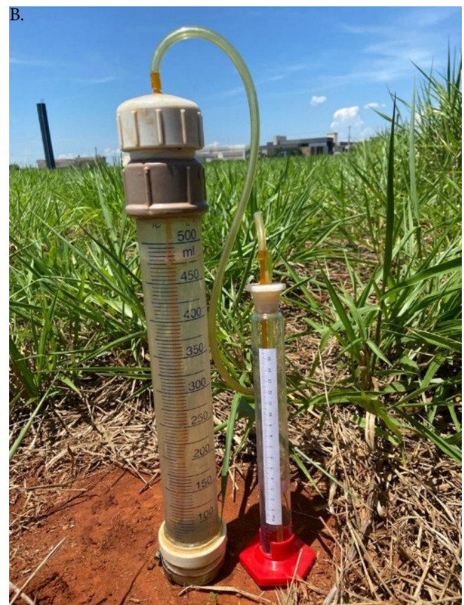
Figure 1. Scheme of the alternative tension infiltrometer (A) and the tension infiltrometer built in operation (B)
